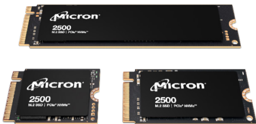
Micron 2500 NVMe SSD (M.2 form factors: 22 x 80mm, 22 x 42mm, 22 x 30mm)
